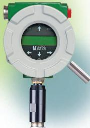
VorTek Instruments' Pro-V™ multivariable flowmeters utilize three primary sensing elements—a vortex shedding velocity sensor, an RTD temperature sensor, and a solid-state pressure transducer—to measure the mass flow rate of gases, liquids and steam. Because the Pro-V™ is able to measure all process variables within a single device it provides exceptional accuracy, simplifies system design and reduces installation costs.
