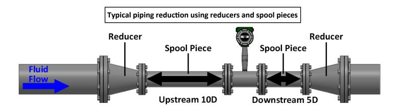
M24R Reduced Bore Vortex with integrated reducing flanges
