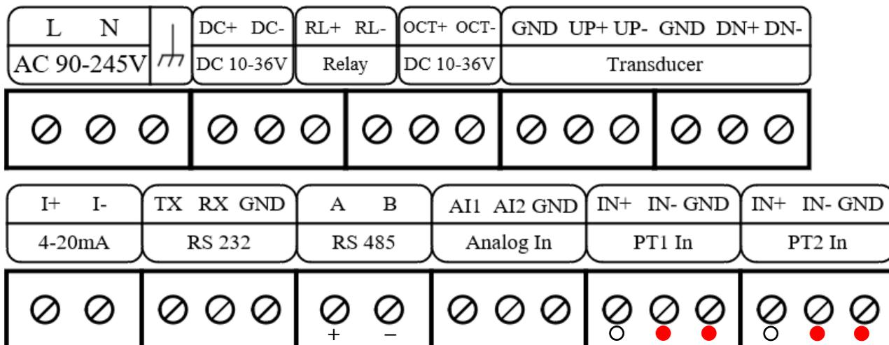
For double-shielded transducer cable: "-" on Blue wire, "+" on Brown wire, and "shield" on Black shield wire.
