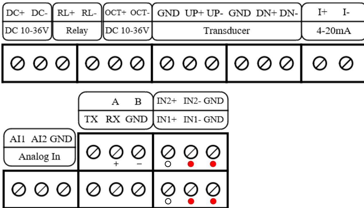
For double-shielded transducer cable: "-" on the Blue wire, "+" on the Brown wire, and "shield" on the Black shield wire.
